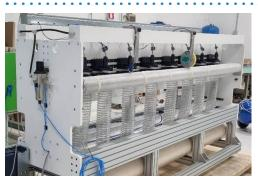
This is a **FAST AND STABLE DEVICE** designed to punch **MACRO HOLES** of various diameters and shapes in **MOVING MATERIAL** and in particular, it works with **PLAIN OR PRINTED FILM**. This model has to be integrated into existing machinery such as extruders, slitters, bag machines etc. It is suitable to make holes on fruits and vegetables bags, garbage bags, paper bags, foam etc.
